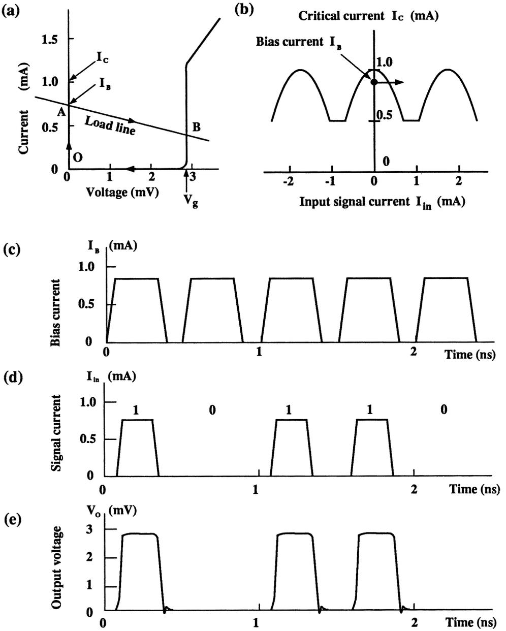
Fig. 3 Computer-simulated JIL gate switching. (a) I-V characteristics. (b) Threshold characteristics. (c) Bias current. (d) Input signal current. (e) Output voltage.
