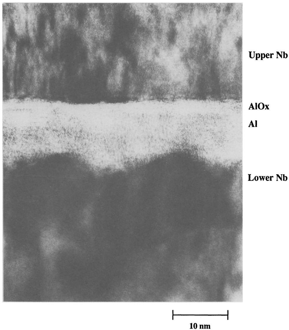
Fig. 5 Cross sectional TEM image of Nb/AlO<sub>x</sub>/Nb junction, where AlO<sub>x</sub> consists of aluminum oxide formed on a sputter-deposited thin aluminum layer.
