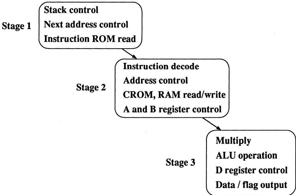
Fig. 19 Three-stage DSP pipelining.
