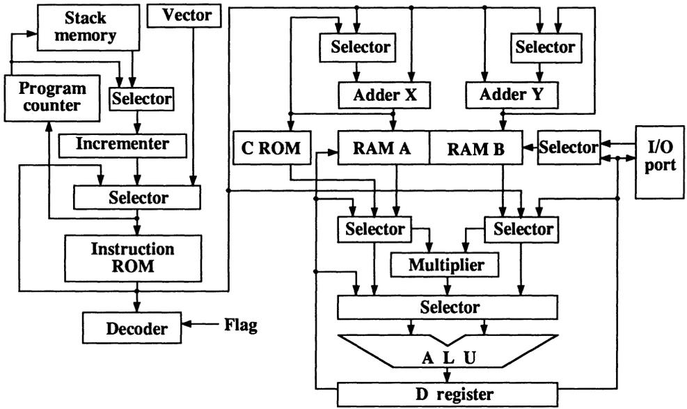
Fig. 18 Eight-bit DSP schematic.
