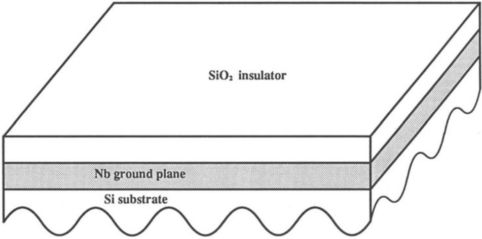
(a) Ground plane and insulating layer deposition
