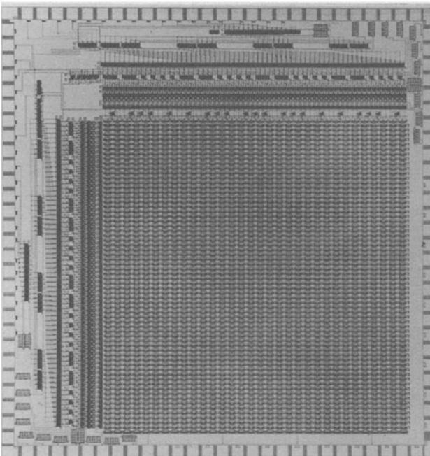
Fig. 21 (Left) Four-kbit memory chip, measuring 7.7 x 7.7 mm.
