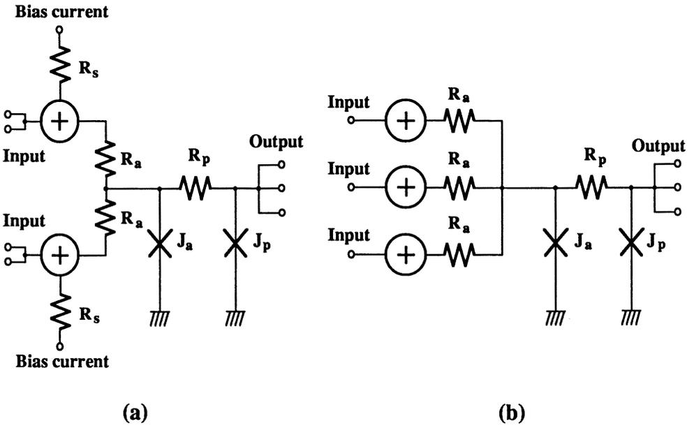
Fig. 10 Equivalent circuits. (a) 2OR-AND (unit cell) gate. (b) 2/3 MJ gate.
