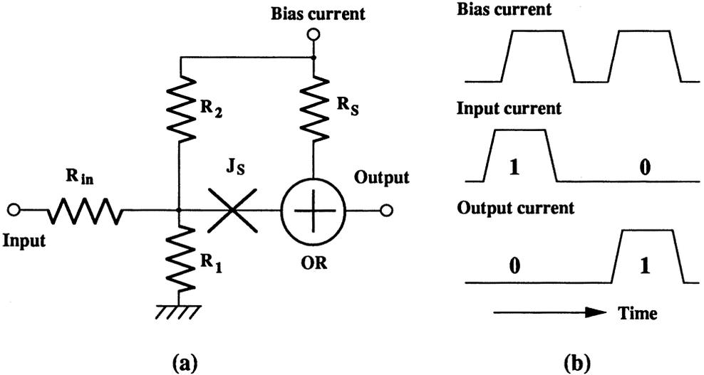
Fig. 11 Timed inverter gate. (a) Equivalent circuit. (b) Timing sequence.
