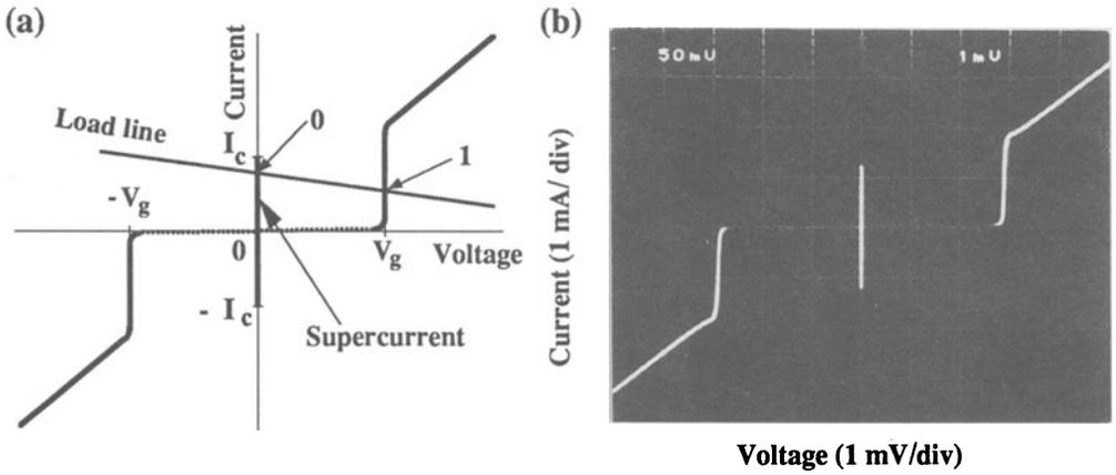
Fig. 1 Josephson junction I-V characteristics. (a) Schematic. The bold central line shows supercurrent. (b) Actual oscilloscope I-V curve for a typical junction.
