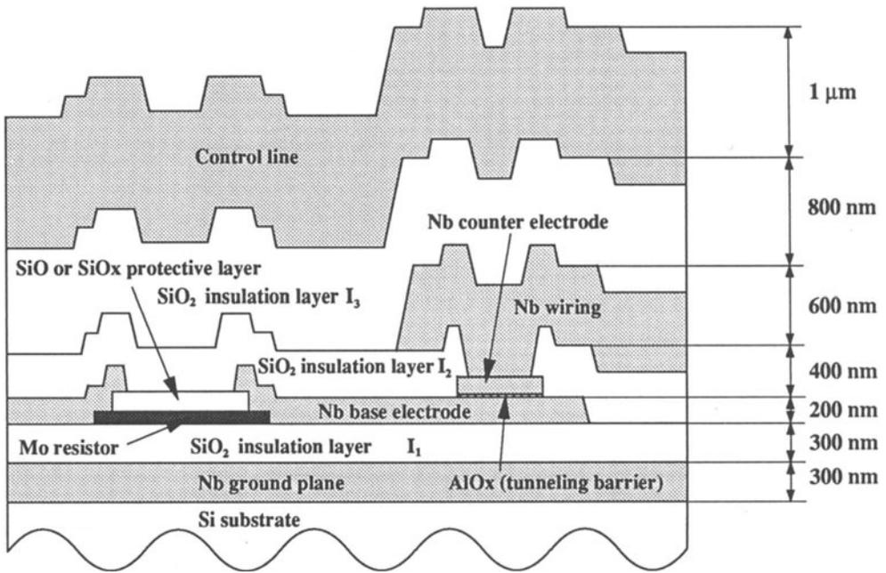
Fig. 6 Typical Josephson circuit with Nb/AlO<sub>x</sub>/Nb junctions.
