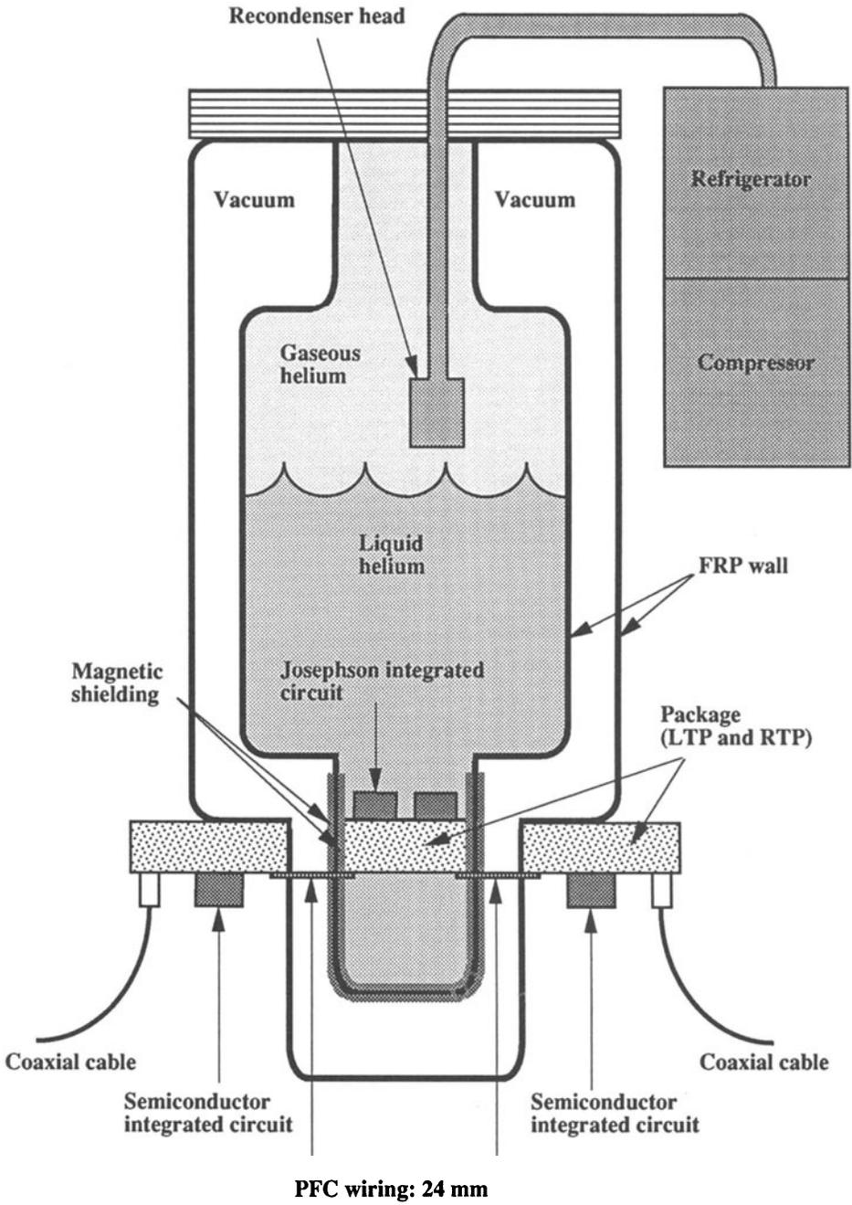
Fig. 23 Cryostat cross section.
