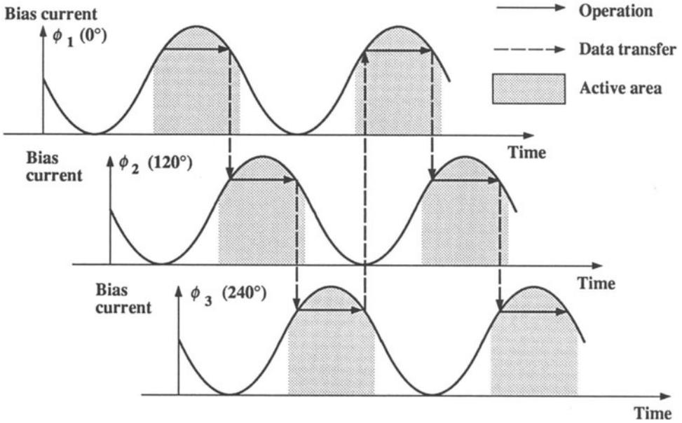
Fig. 13 Logic operation with a three-phase sinusoidal power supply.
