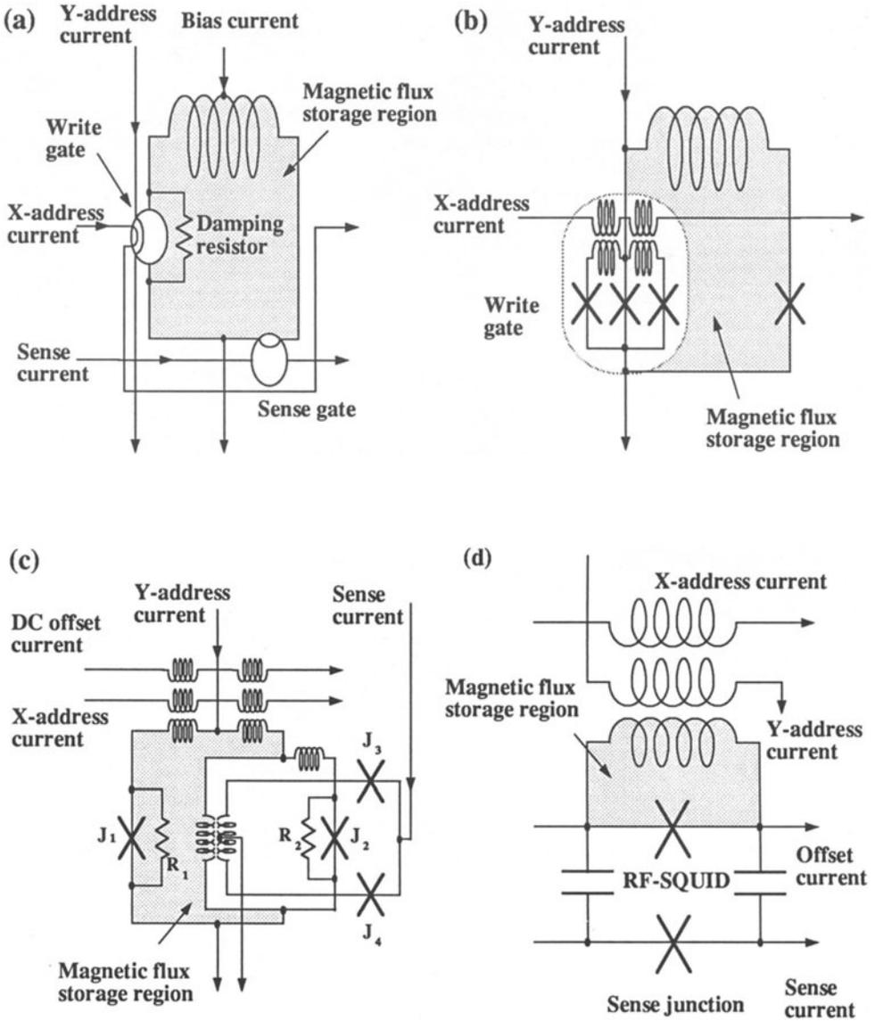
Fig. 4 Equivalent circuits for Josephson memory cells. (a) Conventional Henkels type. (b) Variable threshold. (c) Vortex transition. (d) Capacitively coupled.
