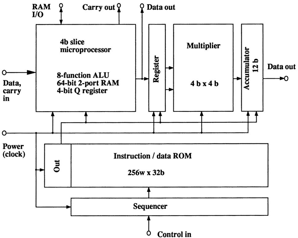
Fig. 16 Four-bit processor schematic.
