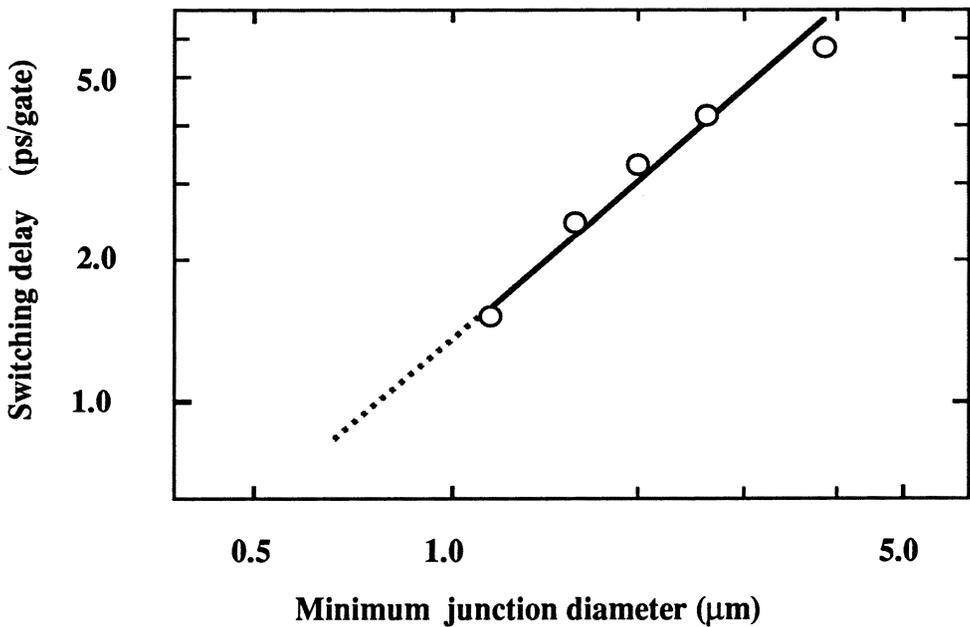
Fig. 9 Fastest gate delay and minimum junction diameter.
