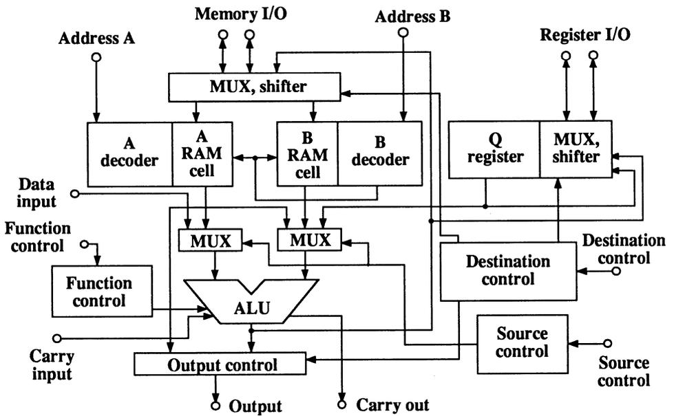
Fig. 14 Four-bit microprocessor schematic.
