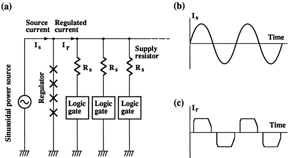
Fig. 12 Conventional power system. (a) Circuit diagram. (b) Current waveform from a sinusoidal current. (c) Current waveform from a regulator.
