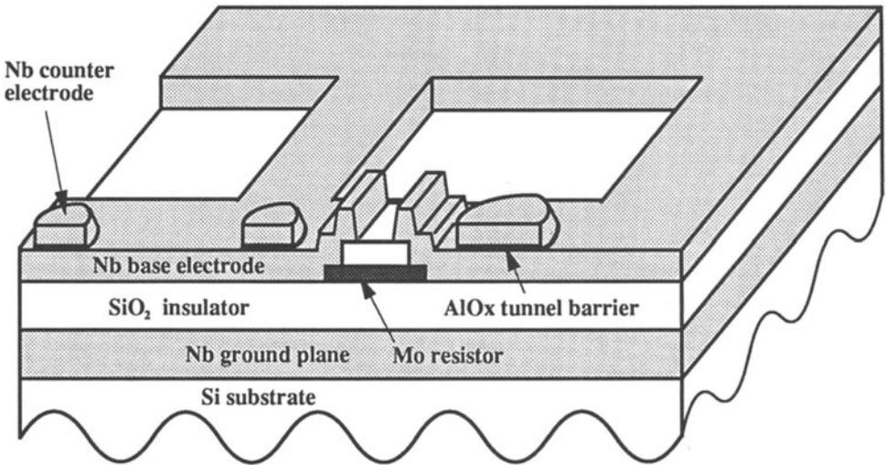
(b) Deposition and patterning of resistor and junction
