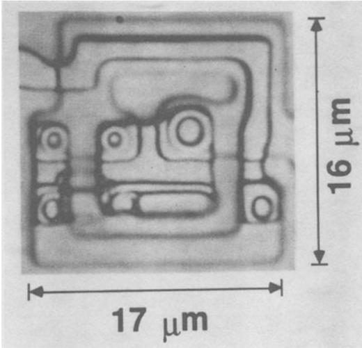
Fig. 7 (a) (Left) MVTL OR gate with a minimum junction diameter of 1.2 μm. (b) (Below) Gate cross section. Doughnut-like structures are Nb/AlOx/Nb junctions. Here, the minimum junction diameter,  $J_1$  is 1.2 μm in the case of the gate in (a), but it is typically 1.5 to 2.5 μm for the actual circuits.
