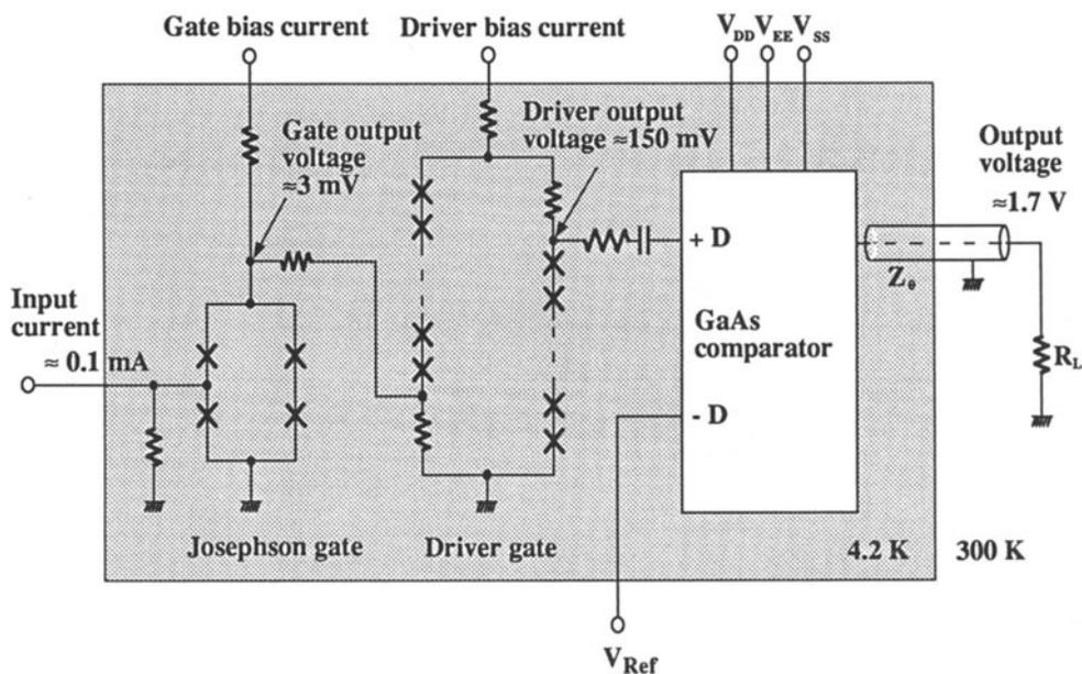
Fig. 22 Equivalent circuit for testing an output interface consisting of a 4 JL Josephson gate, a driver gate, and a GaAs comparator.
