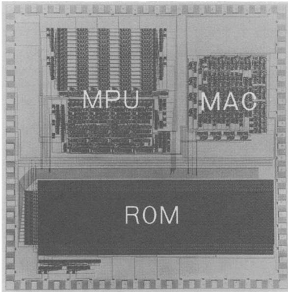
Fig. 17 (Left) Four-bit processor chip, measuring 5 x 5 mm.
